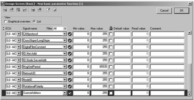
The table below defines the allowable values for each of the *Sensor's* parameters that can be modified using the PLUS+1 Service Tool.
